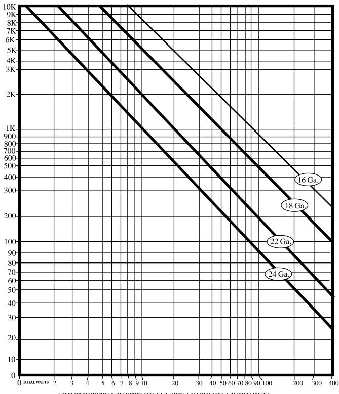
ADD THE TOTAL WATTS OF ALL SPEAKERS ON A WIRE RUN.
